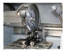
The **Flange Mounted Motor** is supported on a cross shaft with four bearing mounts for stable and accurate cutting
