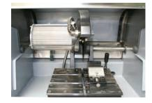
Wide open work area incorporates a large **T-slot Table** with replaceable top plates
