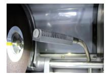
The optional **LED Task Light** is easy to position to provide optimal illumination
