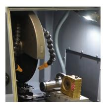
Long life **LED Light** illuminates the cutting chamber
