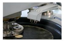
Exact droplet dosing with reverse rinsing function keeps lines clear and ready for use
