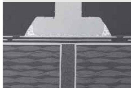
PCB cross section with soldered pin
