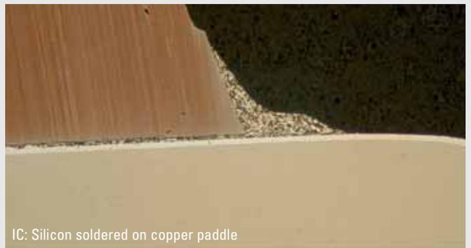
IC: Silicon soldered on copper paddle
