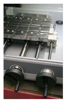
Integrated Z-axis and automatic cross feed table make thin cuts possible.
