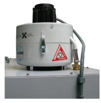
Optional **Mist Extractor** keeps cutting chamber clean and aids in clear visibility of cutting operation
