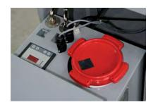
Optional **Recirculation Coolant System** maintains constant water temperature with refrigeration coils
