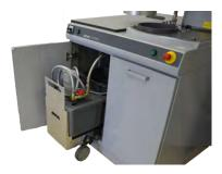
A unique, dual chamber **Recirculation System** preserves coolant and fits perfectly in the **SystemLab** cabinet
